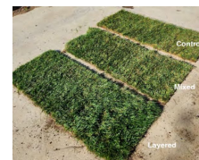
Sod with engineered soil
